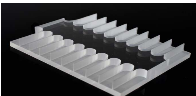
Figure 16: Scanning mirror with lightweight structures on the rear side
