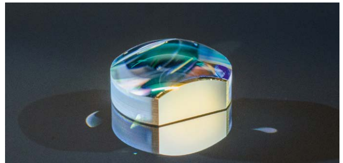
Figure 17: Solderable coating on the side of a lens
