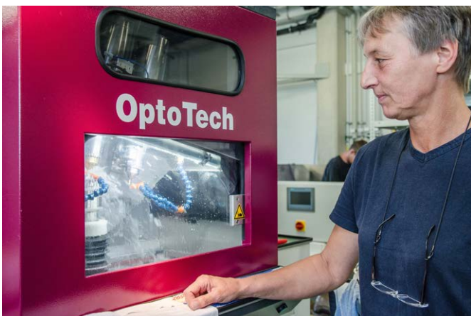
Figure 7: Grinding process on CNC machine
