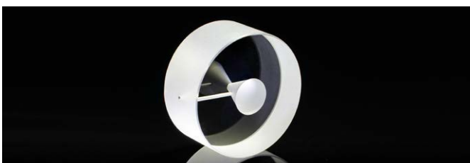
Figure 4: Substrate with conical hole, produced by ultrasonic drilling
